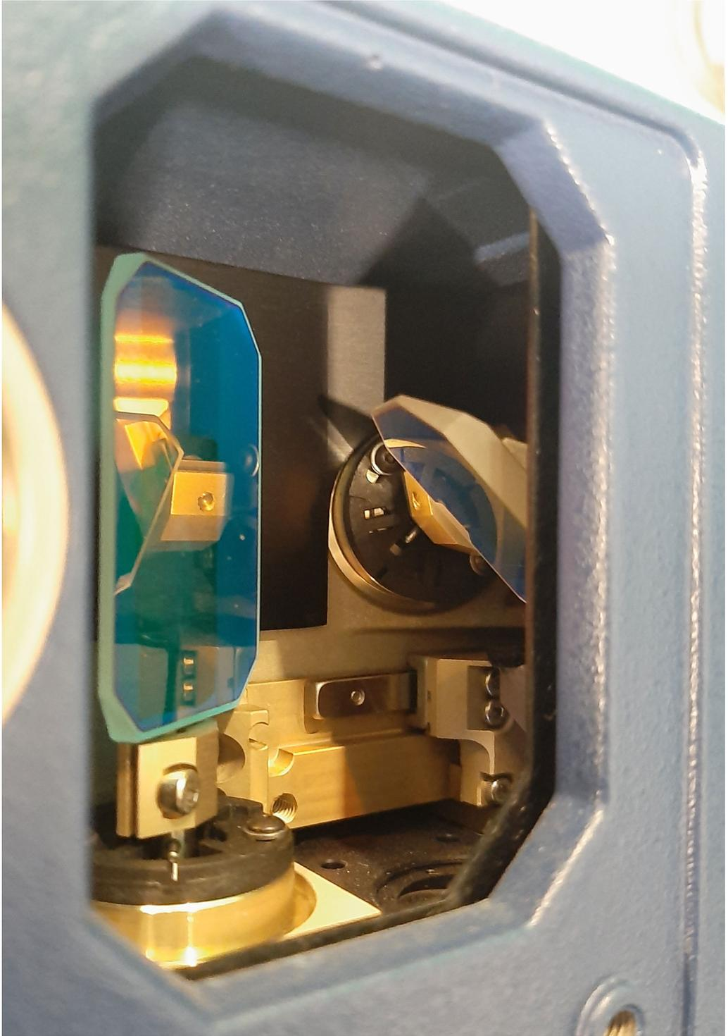
Figure 3.1: The two rotating mirrors inside a vibrometer.
