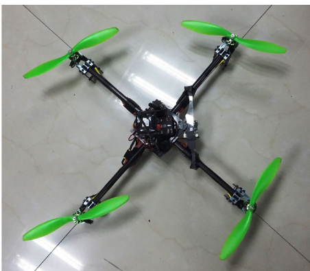
FIGURE 3 Quadrotor experimental setup of 6DOF [Colour figure can be viewed at wileyonlinelibrary.com ]
