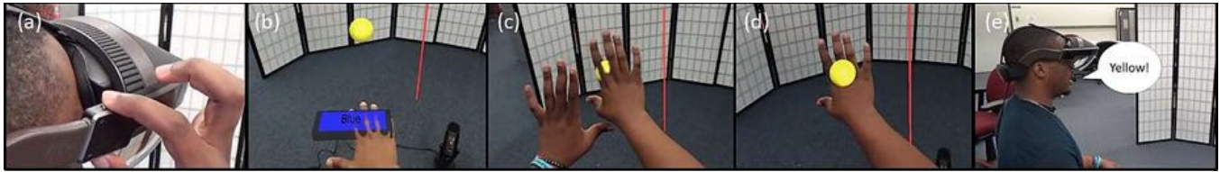
Figure 2: The five mode switching techniques used: (a) hardware button, (b) virtual button, (c) non-preferred hand, (d) depth, and (e) voice.
