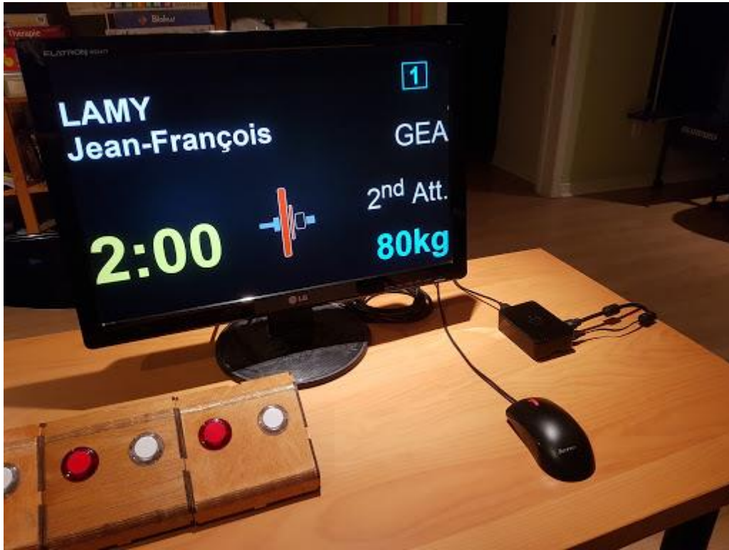
Figure 7: Raspberry Pi3B used as display with Bluetooth refereeing devices
