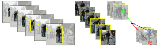
Fig. 9: After tracking, the video data is normalized by scale and position of the human. The normalized action tracks are used as input data for the action recognition.
