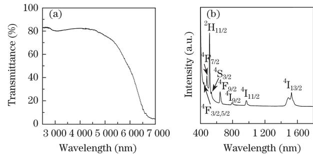
Fig. 1. (a) IR transmittance spectrum and (b) absorption spectrum of  $\text{Er}^{3+}$ -doped bismuth germanate glass.
