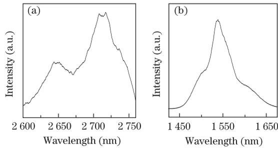
Fig. 2. IR emission spectrum at (a) 2.7 and (b) 1.5  $\mu\text{m}$  of  $\text{Er}^{3+}$ -doped bismuth germanate glass.
