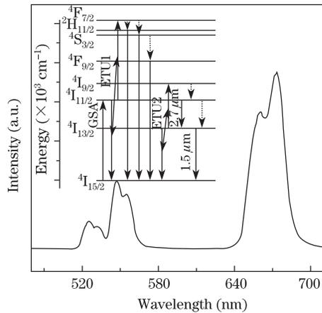
Fig. 3. Upconversion spectrum of  $\text{Er}^{3+}$ -doped bismuth germanate glass. (Inset) Energy-level diagram of  $\text{Er}^{3+}$  pumped by 980 nm.
