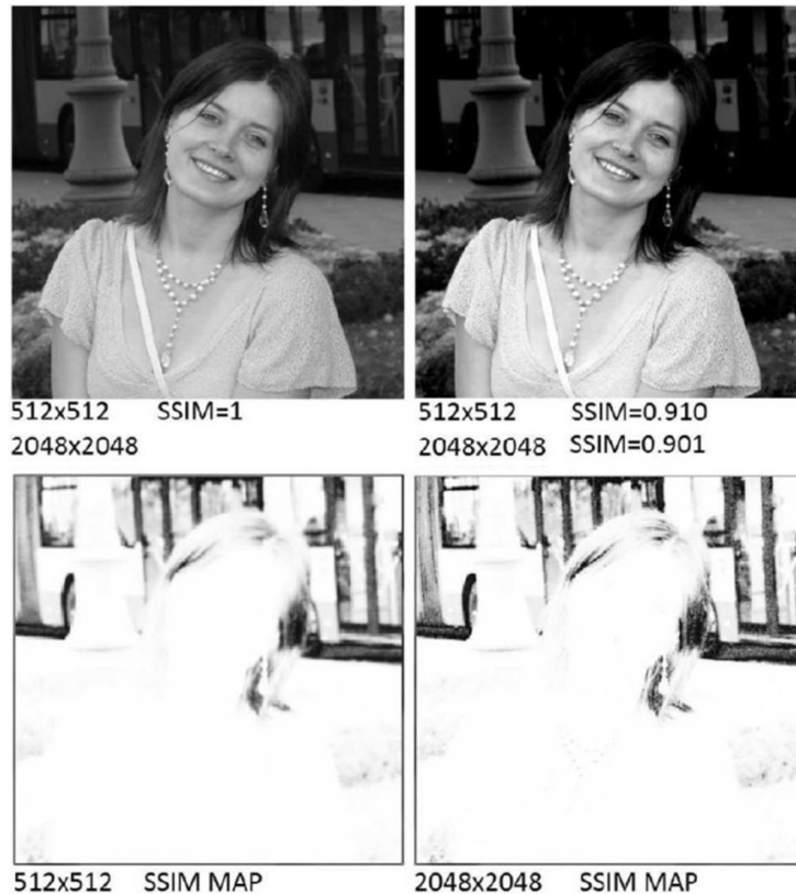
Fig. 4. The image distorted by increasing the contrast and the SSIM maps of the different size images, obtained by Algorithm 2 .
