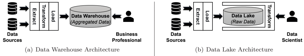
Fig. 1. Comparison of the Data Warehouse Architecture and the Data Lake Architecture.
