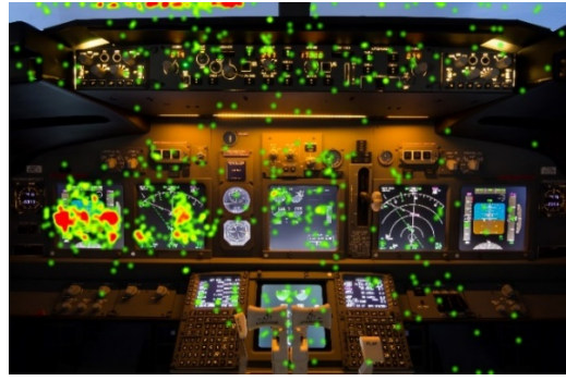
Fig. 11 b - Heatmap of a landing with an engine failure
