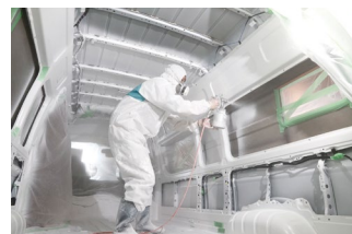
Spray coating achieving superior insulation
