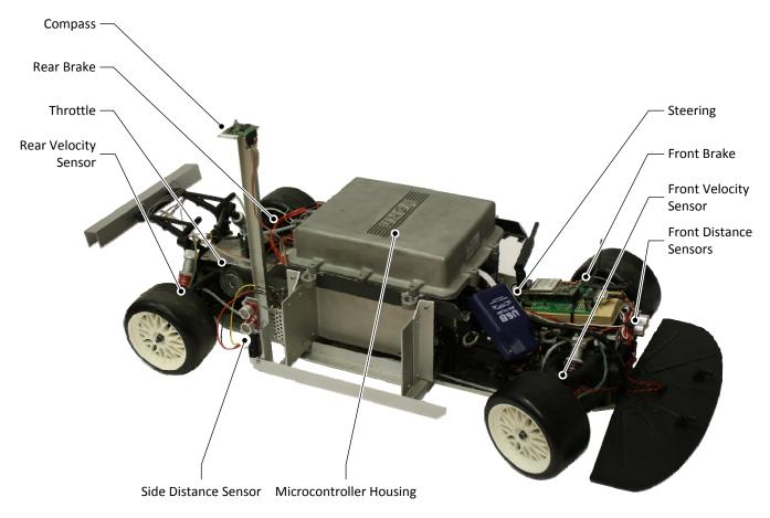
Fig. 5. The model car of the VeRa Rapid Control Prototyping platform.
