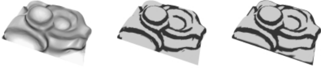
Figure 1: Left: Maximal curvature on a technical model, dark regions denote high curvature. Prefiltering by a median filter has been applied. Middle: After thresholding. Right: After an opening and a closing operation. The mesh boundary was added to the feature. Visual artifacts arise from color interpolation over large triangles.
