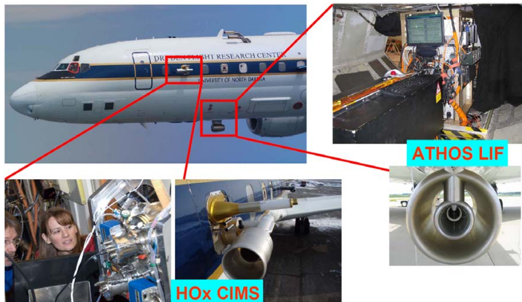
Fig. 1. Pictures showing the setup of the LIF and CIMS instruments for OH and HO 2 measurements on the NASA DC-8 aircraft during ARCTAS 2008.
