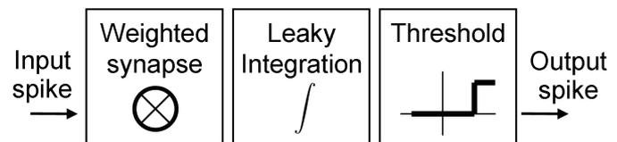
Fig. 1. Block diagram of a leaky-integrate-and-fire neuron.
