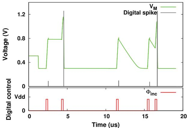
Fig. 3. Analog simulation: Evolution of membrane potential, neuron output, and control signals.
