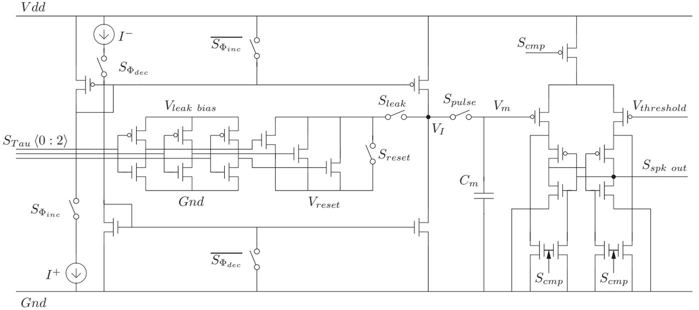
Fig. 2. Analog LIF neuron schematic
