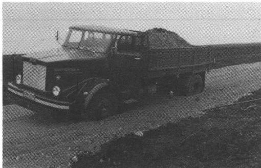
Fig. 1. Technical problem with heavy counterweight on a road with low bearing capacity.
