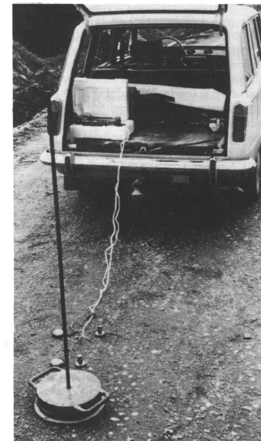
Fig. 3. Light seismic bearing capacity measurement system.
