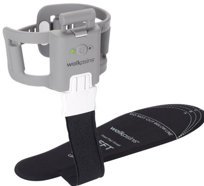
791 792 Figure 1. Picture of the Walkasins sensory neuroprosthesis device showing the pressure sensor embedded Foot Pad that 793 is placed in the subject's shoe and connected to the Leg Unit that houses an embedded microprocessor with software, 794 supporting electronics, a rechargeable battery, and four tactile stimulators placed around the lower leg. The system is 795 worn bilaterally. Leg Unit and left Foot Pad shown
