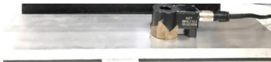
Figure 11. Flat plate sliding scanning method of probe.
