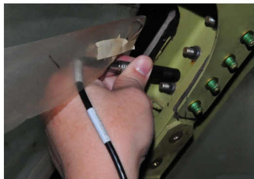
Figure 10. Scanning method of sliding hole edge.
