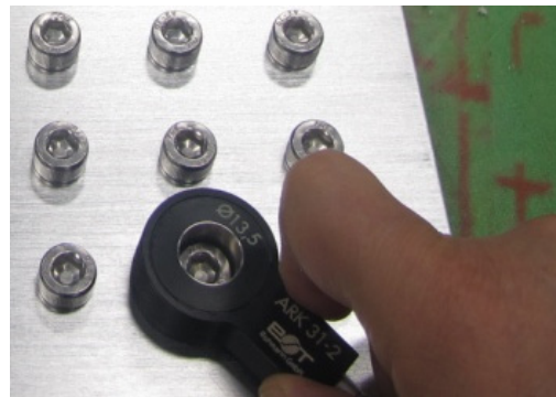
Figure 9. Scanning method of circular nail hole.
