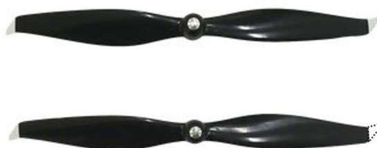
Figure 8. The damaged propellers used in the experiments.
