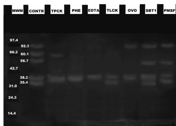
Figure 4. SDS-PAGE zymogram of alkaline digestive proteases of Cichlasoma beani : Molecular Weight Marker (MWM), rabbit phosphorylase B (97.4 kDa), bovine serum albumin (66.2 kDa), ovalbumin (42.7 kDa), carbon anhydrase (31.0 kDa) and lysozyme (14.4 kDa); control (without inhibitor); inhibitors were the same as in Figure 3.
