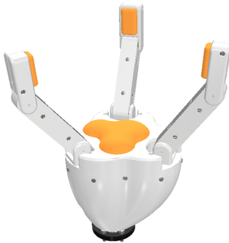
Figure 1. Open-source 3D Printed Three-Fingered Robotic Gripper.
