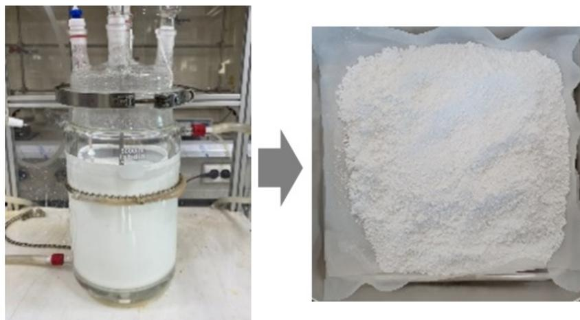
**Figure 10.** Photographs of the reactor used for the suspension polymerization of PAN polymers (**left**) and the obtained product powders (**right**).
