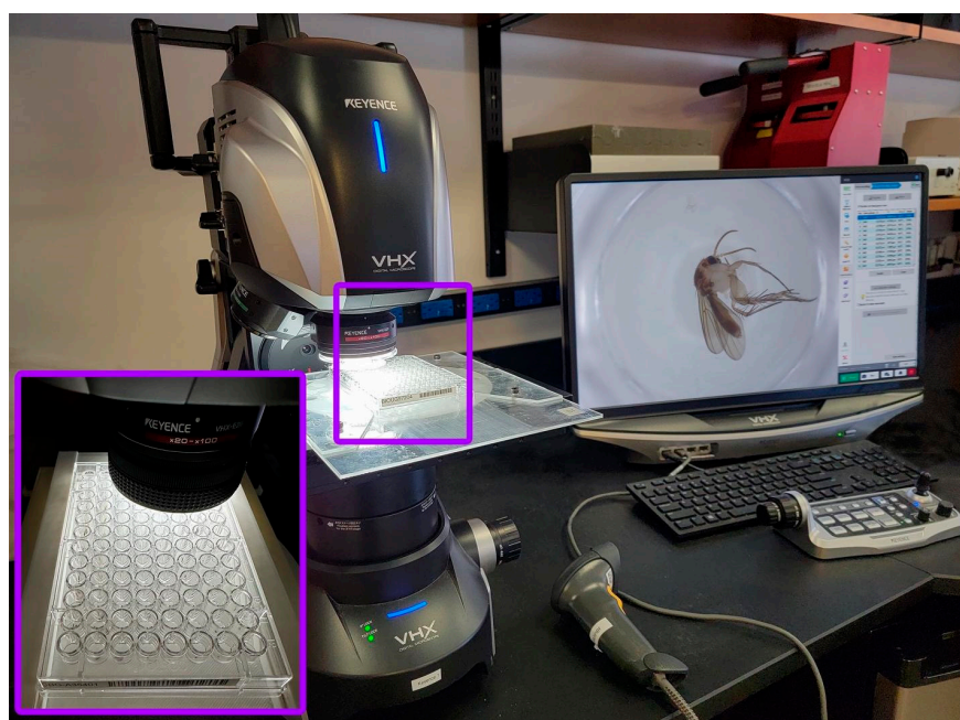
Figure 1. Keyence VHX-7000 Digital Microscope system. The inset shows a microplate within the custom-engineered mount.
