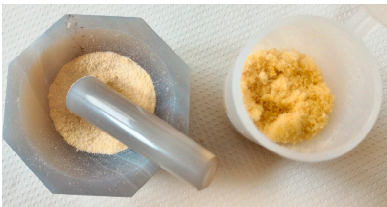
Figure 4. Sample of lyophilized pectin powder from the WOP1 test (right), which was ground in a quartz mortar (left) prior to the diffuse reflectance infrared Fourier transform (DRIFT) experiments.
