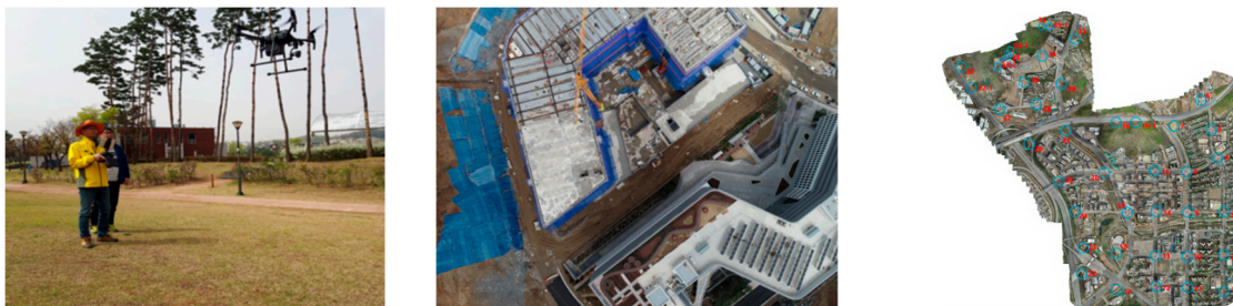
(a) Operation of UAV (b) Outcome of the orthoimage shooting (c) 35 GCPs for picture matching and position correction
