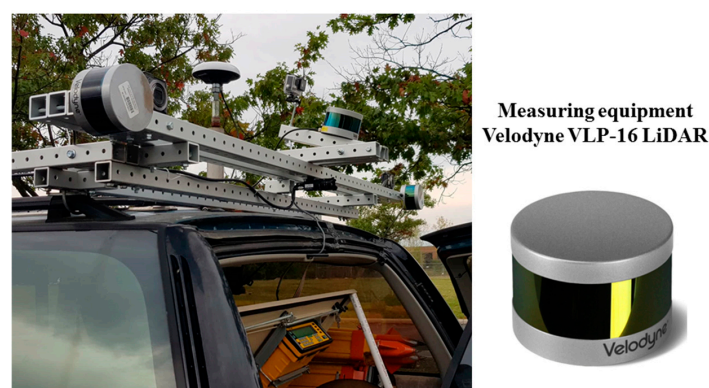
Figure 5. Rear view of the platform equipped with Velodyne VLP-16 LiDAR scanner.
