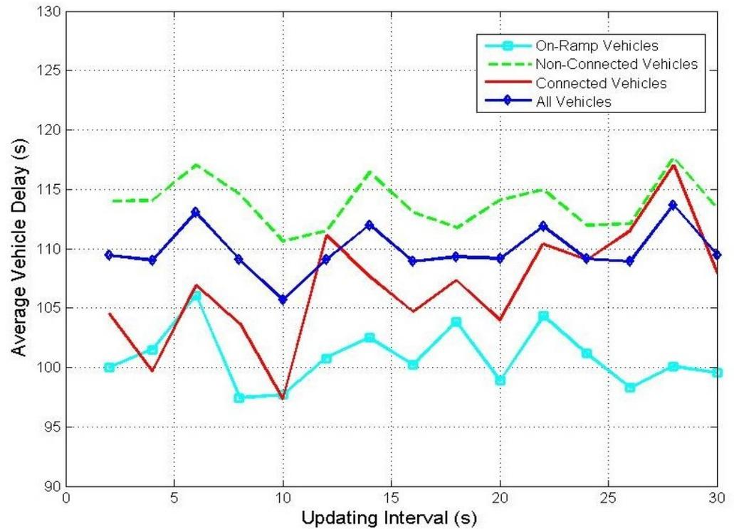
Figure 6. Average delay under different updating intervals.
