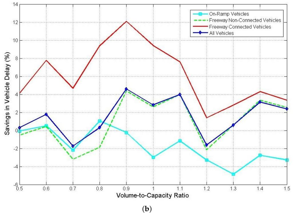
**Figure 8.** Delay savings under different freeway V/C ratios: (a) incident on the right two lanes; (b) incident on the middle two lanes.
