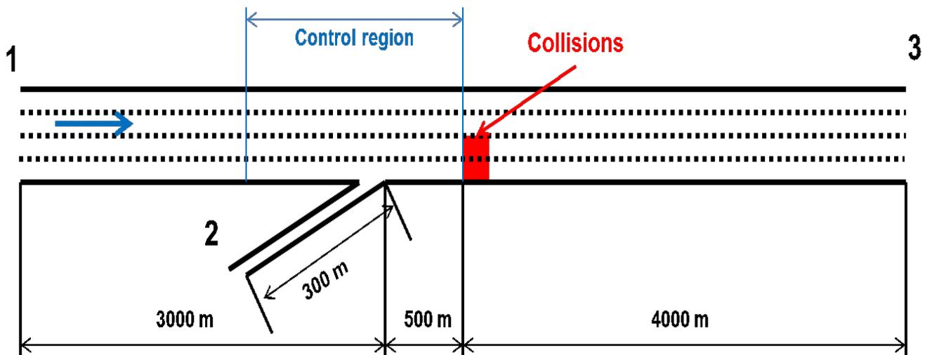
Figure 2. Network geometry (Traffic is loaded from Origins 1 and 2 to Destination 3).
