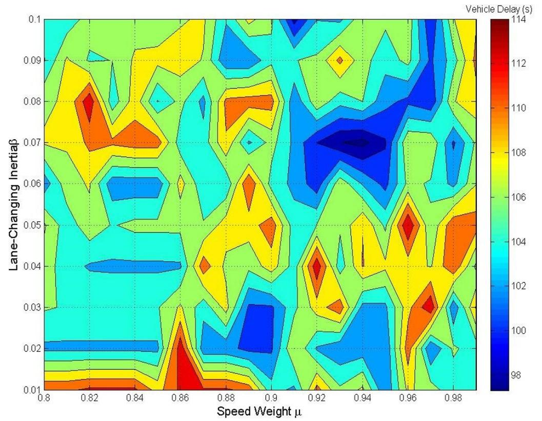
Figure 3. Average delay of CVs under different speed weights and lane-changing inertial factors.
