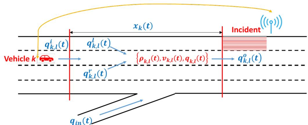
Figure 1. Traffic states at the upstream of one road incident.
