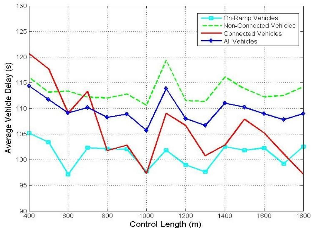
Figure 5. Average delay under different control lengths.
