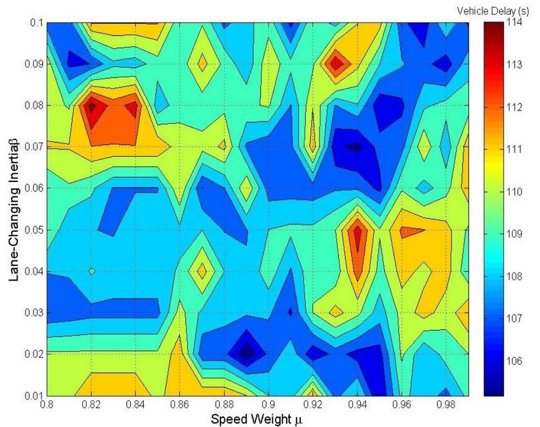
Figure 4. Average delay of all vehicles under different speed weights and lane-changing inertial factors.
