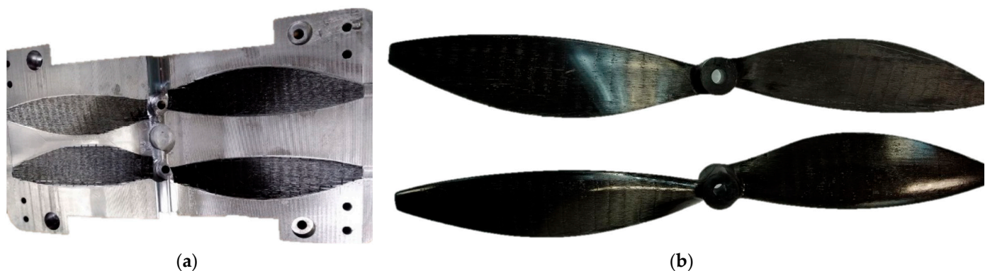
Figure 15. (a) Injection mold for the manufacture of the propellers; (b) manufactured propellers.
