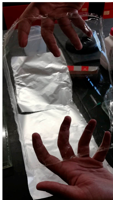
Figure 1. Film obtained by casting method.
