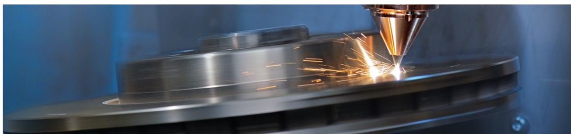
Figure 2. EHLA coating process of a brake disk.
