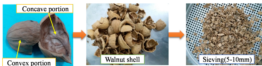
Figure 1. The surfaces of crushed walnut shell and the process of sieving.
