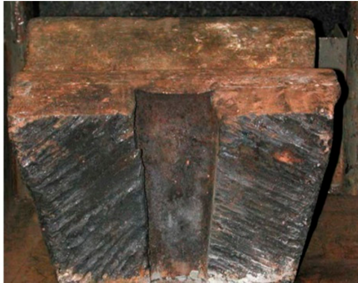
Figure 1. Sample 1. Macroscopic image of the condition of the working surface of the jaw crusher for squashing rocks with a volume of 10–1000 mm. Operating time of about 350 h, throughput of about 80.00 tons.
