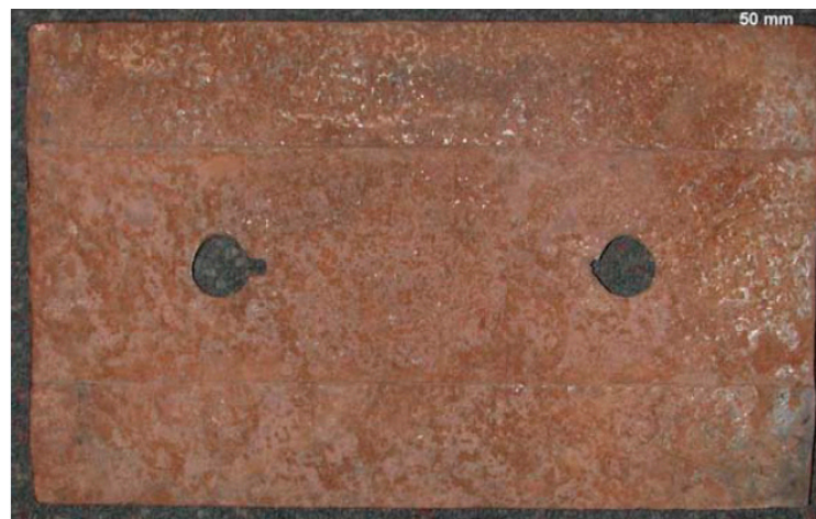
Figure 2. Sample 2. Macroscopic image of the surface condition of the ball mill liner plate covering part of the contracture of the chute. Material volume of 100–1200 mm, throughput of about 200.000 tons.
