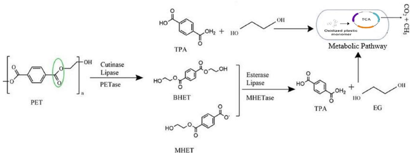
**Figure 6.** Enzymatic degradation mechanism of PET degradation through cutinase, lipase, and MHETase producing terephthalic and ethylene glycol (adapted from [135]).
