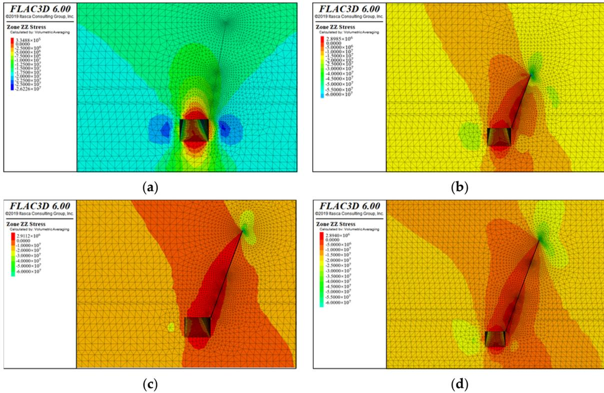
Figure 7. Vertical stress distribution diagram of the roadway with different roof cutting heights: (a) uncut roof; (b) 9 m; (c) 13.5 m; (d) 18 m.
