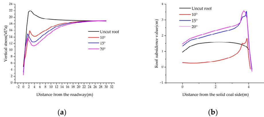
**Figure 5.** (a) Vertical stress curve of the roadway with different roof cutting angles; (b) vertical displacement curve of the roadway with different roof cutting angles.
