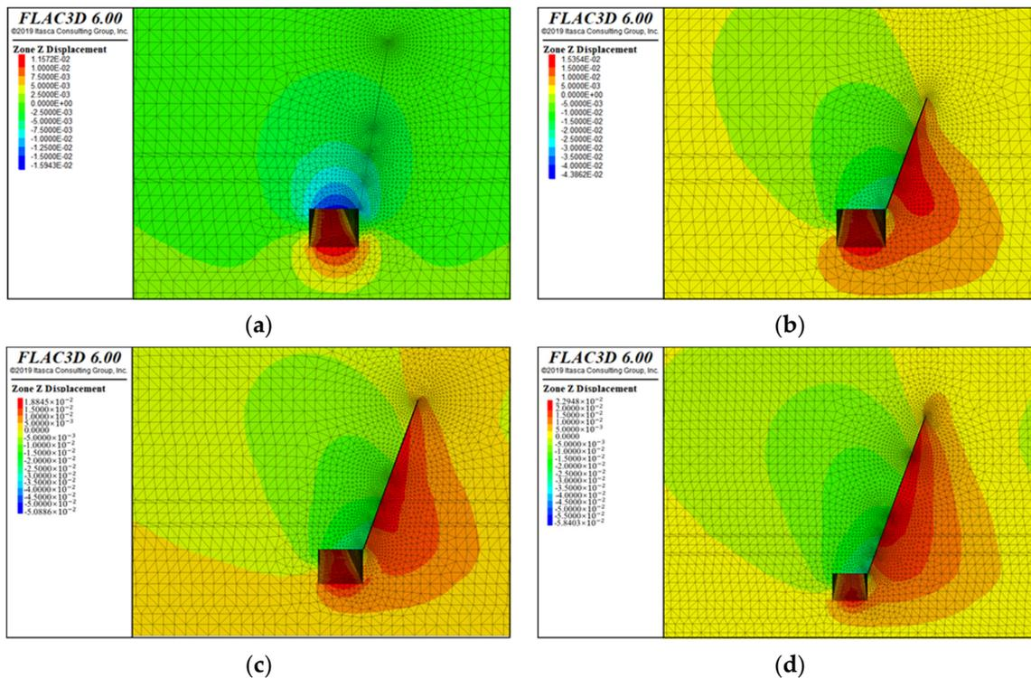
**Figure 9.** Vertical displacement distribution map of the roadway with different roof cutting heights: (a) uncut roof; (b) 9 m; (c) 13.5 m; (d) 18 m.
