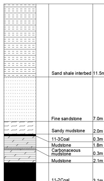
Figure 2. Comprehensive column of the rock strata in the 1127 (1) working face of Guqiao Coal Mine.
