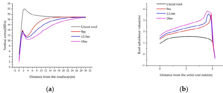
Figure 8. (a) Vertical stress curve of the roadway with different roof cutting heights; (b) vertical displacement curve of the roadway with different roof cutting heights.
