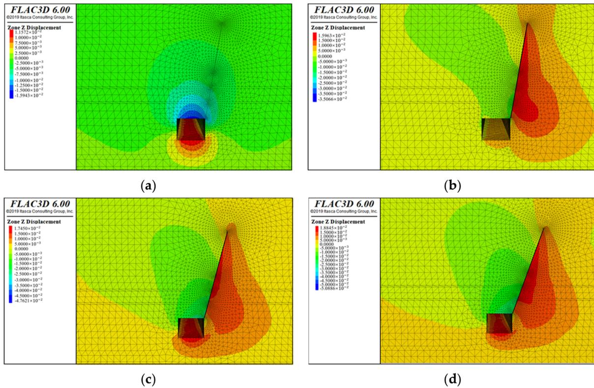
**Figure 6.** Vertical displacement distribution map of the roadway with different roof cutting angles: (a) uncut roof; (b) 10°; (c) 15°; (d) 20°.
