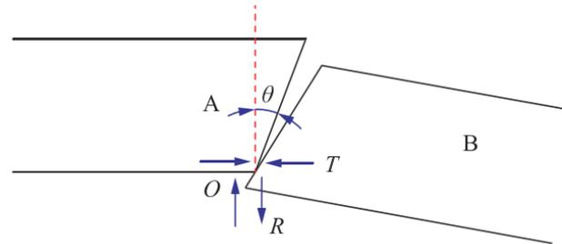
**Figure 3.** Basic roof breaking structure and force analysis by roof cutting and pressure relief.
