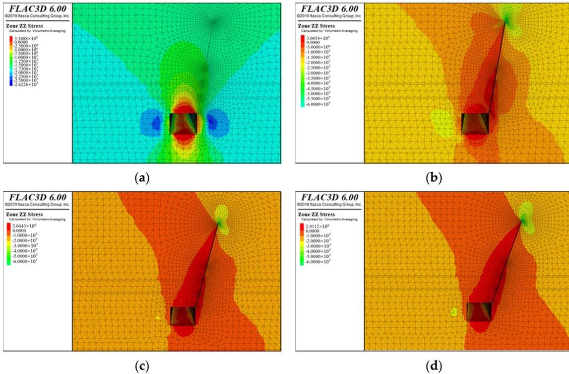
**Figure 4.** Vertical stress distribution diagram of the roadway with different roof cutting angles: (a) uncut roof; (b) 10°; (c) 15°; (d) 20°.
