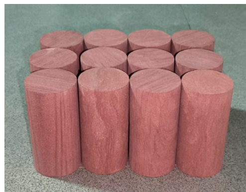
Figure 2. Argillaceous siltstone samples.
