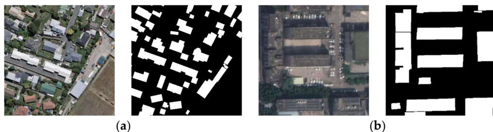
Figure 7. Examples of the images and corresponding labels for the two employed datasets. (a,b) represent the WHU dataset and CHN dataset, respectively. The white pixels stand for buildings.
