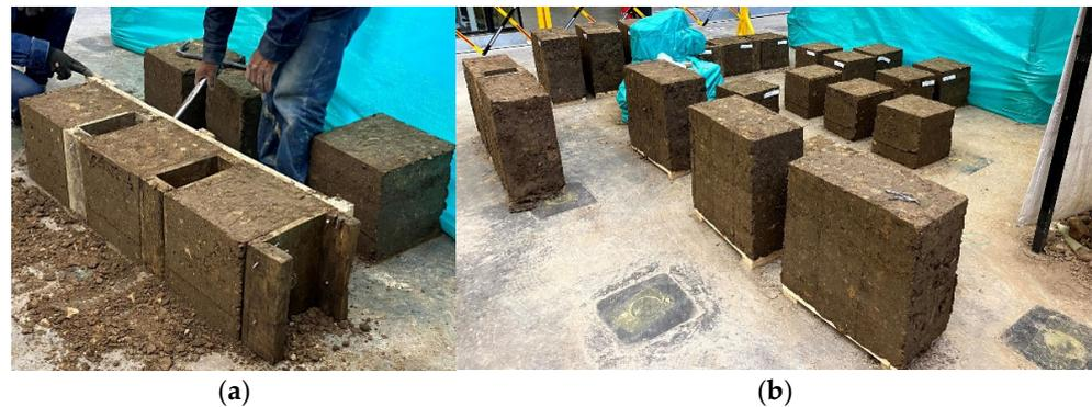
**Figure 7.** (a) RE specimens with dimensions of  $300 \times 300 \times 300$  mm for direct cyclic shear test; (b) compression and shear specimens during drying process.
