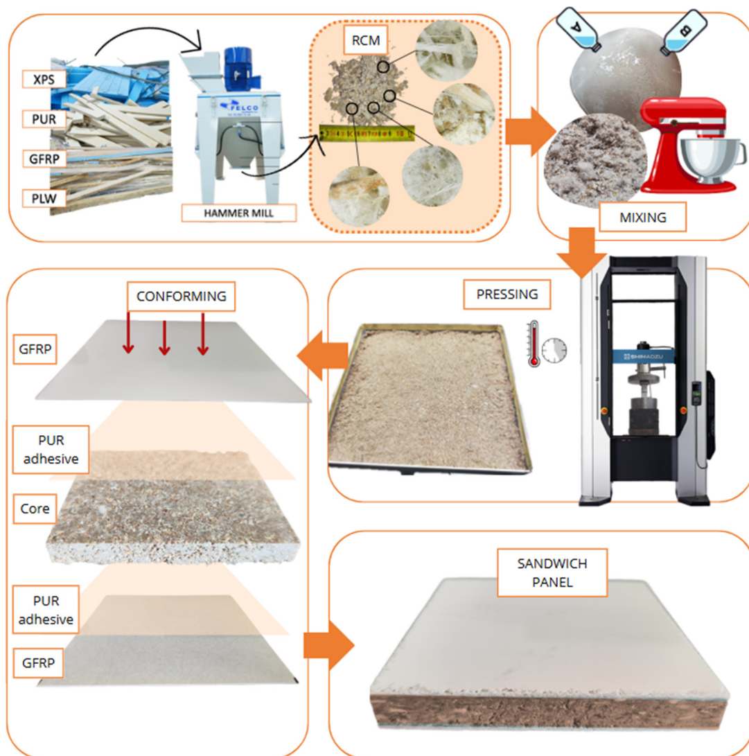
Figure 4. SP-RCM manufacturing process (A: resin, B: hardening agent).
