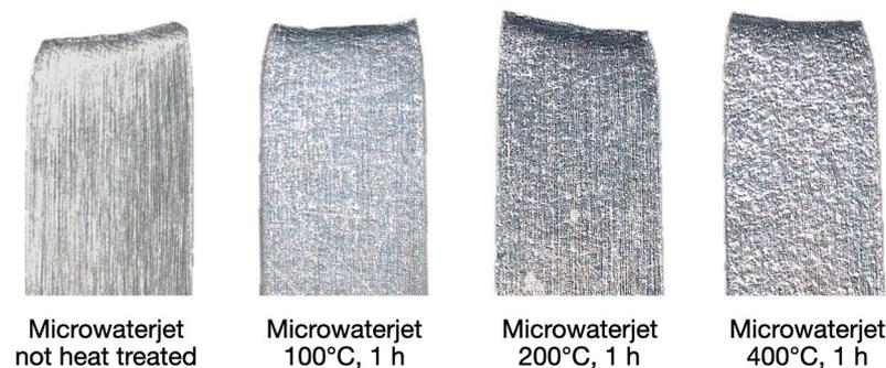
**Figure 16.** Microwaterjet cut EN AW-5005-H24 samples (3 mm in width,  $500 \mu\text{m}$  in thickness) of different annealing conditions, after failure in micro-tensile tests. All samples failed by ductile fracture. Necking occurred in the form of pronounced thickness and width reduction at the fracture site.
