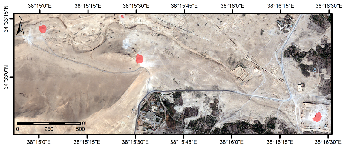
Figure 8. Red: post-processed change map from Figure 7 overlaid on the 2 September 2015 WorldView-2 image reported in Figure 5. All the main damaged areas are correctly identified (©European Space Imaging/DigitalGlobe).
