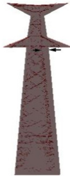
Figure 10. Reconstruction gap caused by pylon inclination.
