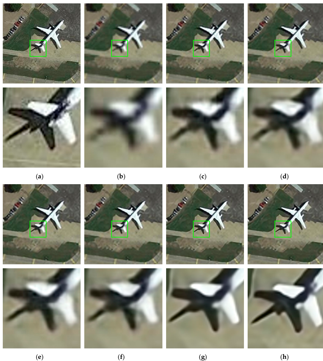
Figure 12. Comparisons of the reconstructed results of 'airplane_035.jpg' with a scale factor of \times 4 for different methods; the values of PSNR and SSIM are given: (a) original, (b) bicubic (25.78 dB/0.8053), (c) SRCNN (27.20 dB/0.8494), (d) FSRCNN (27.69 dB/0.8676), (e) ESPCN (27.32 dB/0.8477), (f) VDSR (28.02 dB/0.8950), (g) SRGAN (27.03 dB/0.8554) and (h) DRGAN (28.48 dB/0.9143).
