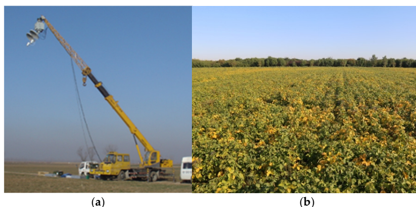
Figure 1. Photograph of the (a) truck-mounted scatterometer system; (b) test site on 9/30.
