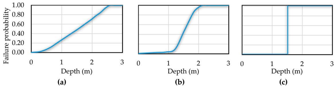
**Figure 5.** Original flooding fragility curves for HV, MV and LV electrical substations and distribution centers (b) (adapted from FEMA, 2009). Softened fragility curve (a) and Hardened fragility curve for sensitivity analysis (c).
