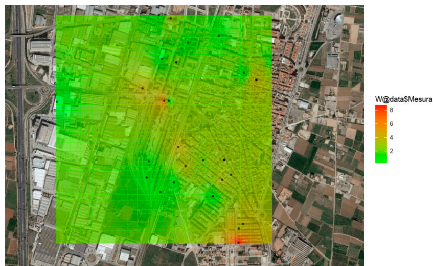
Figure 2. Map of the city of Silla, with the location of the TSs. The color shows the average MF values interpolated with the geostatistical methodology used by our team in the analysis of noise levels [22,23].
