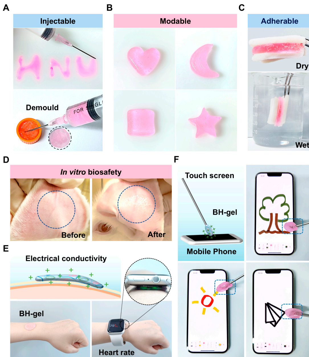
Figure 3. Injectable BH-gel exhibited excellent biocompatibility, deformability, adhesiveness, and electrical conductivity. (A) The injectability of BH-gel using a needle syringe was assessed. (B) Optical images show the moldable features of BH-gel. (C) Photographs showing strong adhesions of the hydrogels with porcine skin in air and under water. (D) The biocompatibility of BH-gel. Representative images of the skin appearance before and after gel application to a rabbit’s ear. (E,F) The electrical conductivity of BH-gel. Demonstration of a BH-gel-based wearable sensor for heartbeat monitoring and a BH-gel-based touchscreen pen used for drawing.
