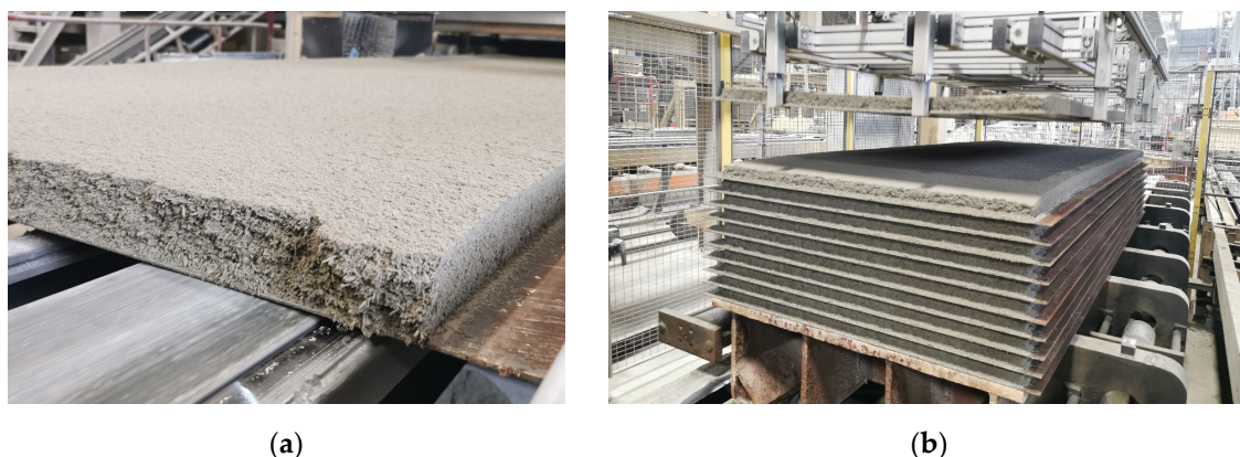
Figure 5. Production of cement-bonded particleboards—CIDEM Hranice, a.s.: (a) layered mixture on a steel pad; (b) layering of individual steel plates with the mixture over each other prior to pressing.
