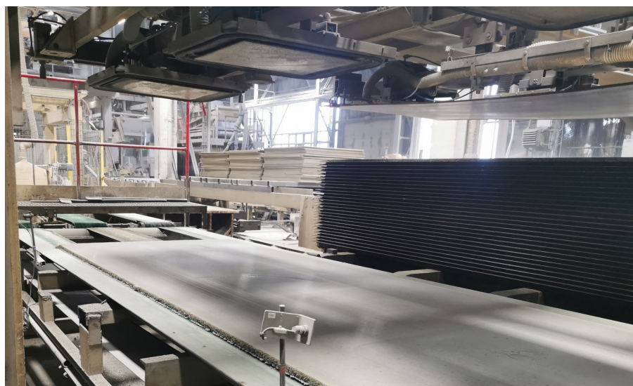
Figure 6. Production of cement-bonded particleboards CIDEM Hranice, a.s.: board after pressing and thermal treatment, before formatting and grinding.
