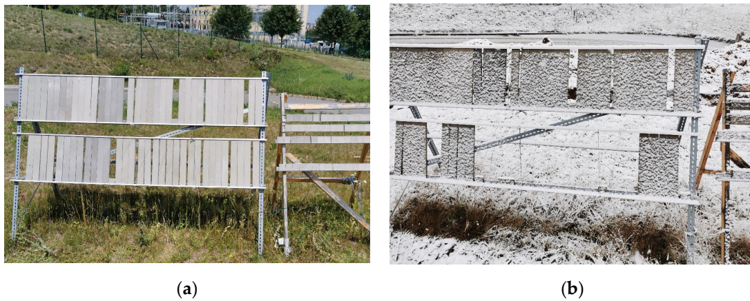
Figure 7. Exposure of test specimens in real climatic conditions over the course of 2 years (Central Europe, Czech Republic): (a) summer 2022; (b) winter 2023/2024.
