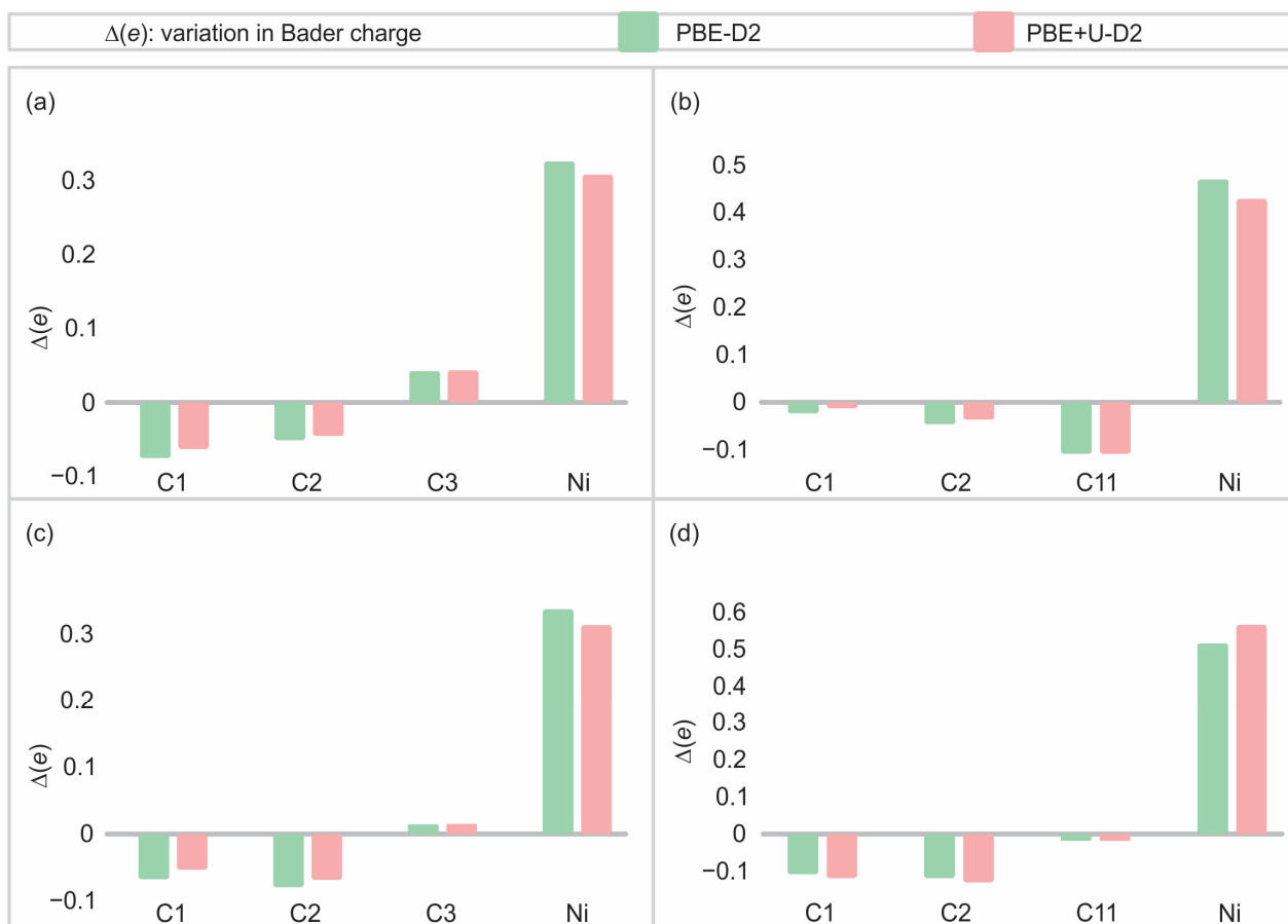
Figure 11. Variation in Bader charges for optimised systems on selected atoms (see Figure 9) before and after Ni adsorption using PBE-D2 and PBE + U-D2 functionals, for the systems: (a) Ni-(6,0) SWCNT, (b) Ni-2vac-(6,0) SWCNT, (c) Ni-(8,0) SWCNT, and (d) Ni-2vac-(8,0) SWCNT.
