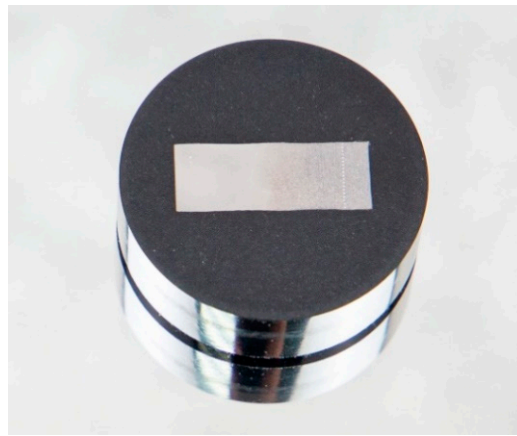
Figure 3. Sample preparation for the microstructure and cross-section analysis.
