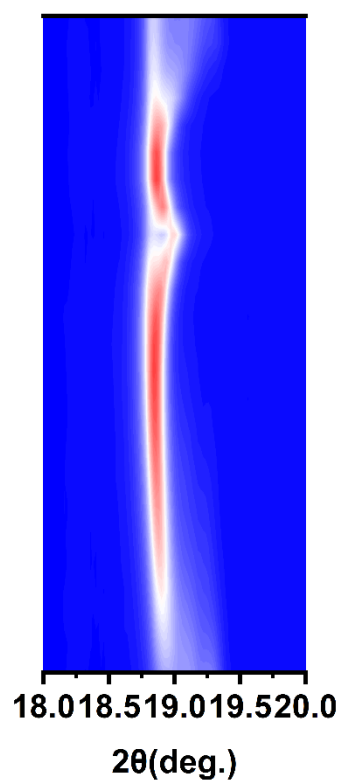
Figure S10. In situ XRD patterns during the first cycle of LCO.
