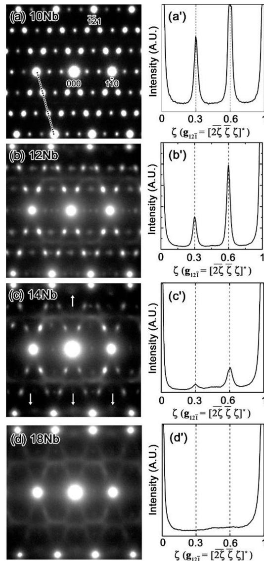
**Figure 3.** Results for Zr-x at.% Nb alloys ( $10 \leq x \leq 18$ ), as obtained by applying the incident beam in the  $[11\bar{3}]$  direction at room temperature: (a–d) diffraction patterns for  $x = 10, 12, 14$ , and  $18$ , respectively; (a'–d') corresponding intensity profiles.
