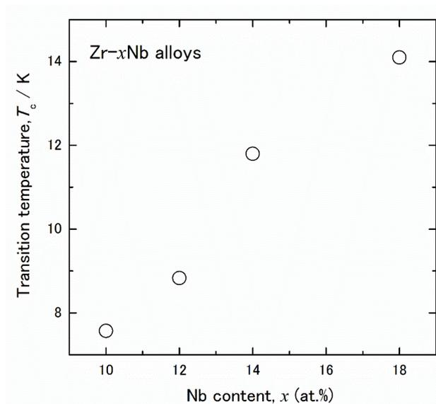
**Figure 2.** Nb content dependence of the superconductive transition temperature ( $T_c$ ) of Zr-x at.% Nb ( $10 \leq x \leq 18$ ) alloys.
